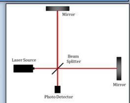
When the beams are in phase, output is maximum.
